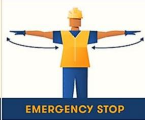
The next two are very important in knowing the difference. The first one, stop, is just to tell the operator to stop whatever action he is doing while other, emergency stop, means that something is wrong and to shutdown.
